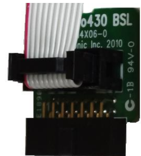
Adapter from 14-pins connection to 10-pins BSL only connection. PN: PE014X06
